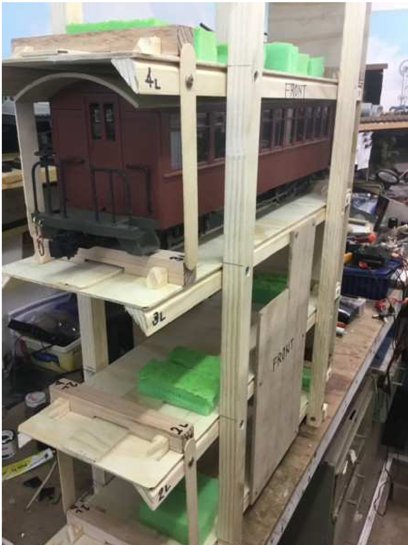
Coach in place, chocked, chocks locked, green foam blocks yet to be positioned.
