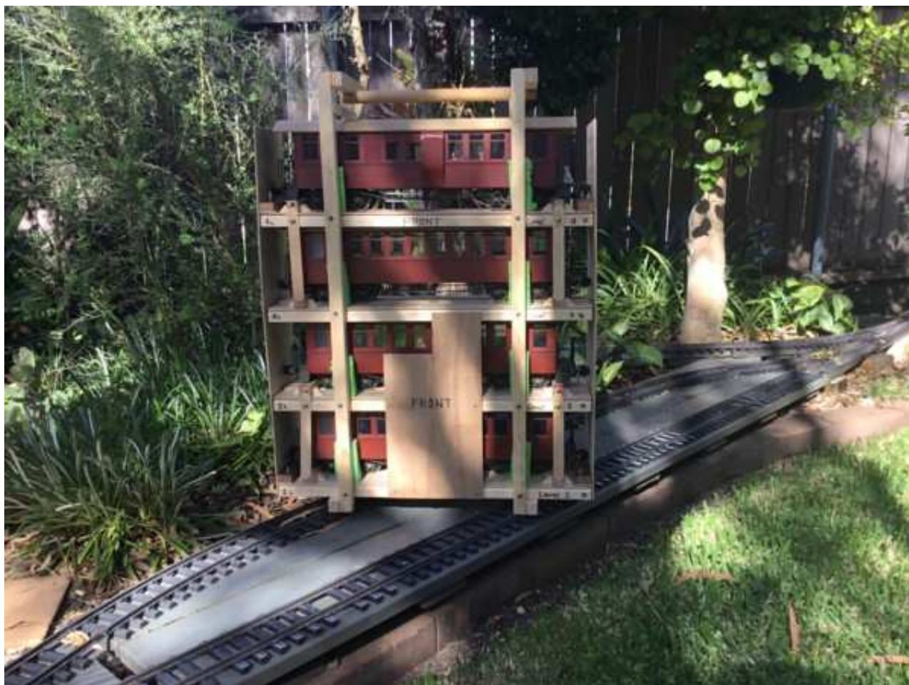
Coaches securely restrained for transit, removable end walls allow quick easy access for withdrawal.
