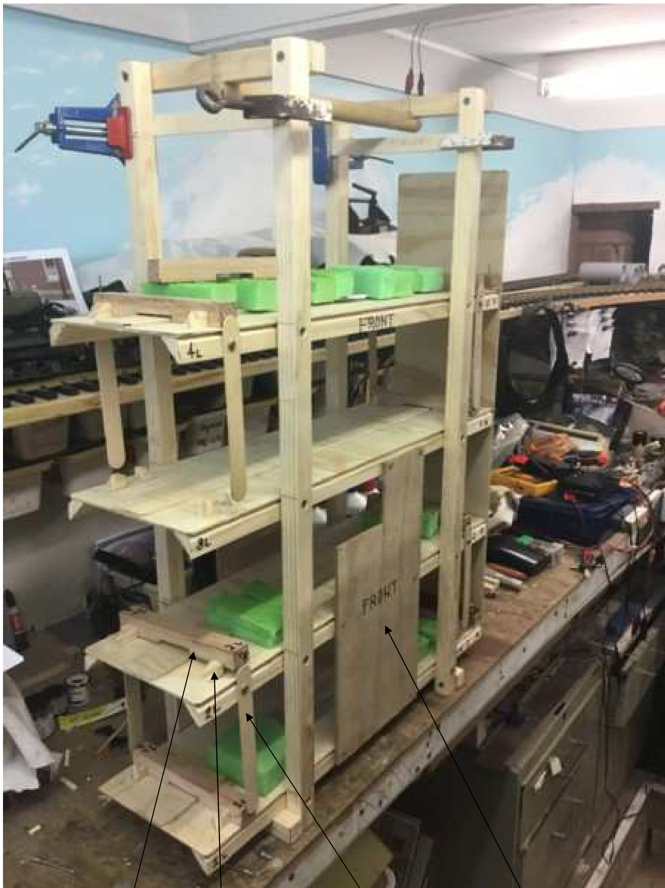
Wheel retainer chocks, chock guides, chock end stop lock paddles, Sheer restraint panel.
